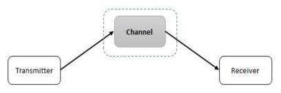
Fig 2.1. Basic elements in a wireless system
