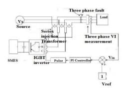
Fig. 4 Schematic diagram of SMES based DVR
