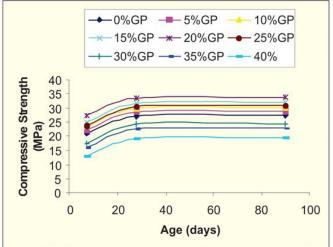
Fig.4. Variation of compressive strength development in concrete
