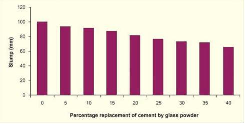
Fig.3. Variation of slump of concrete with cement replacement by glass powder
