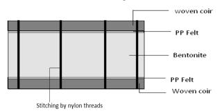
Fig.3.2. Schematic diagram Sample 2
