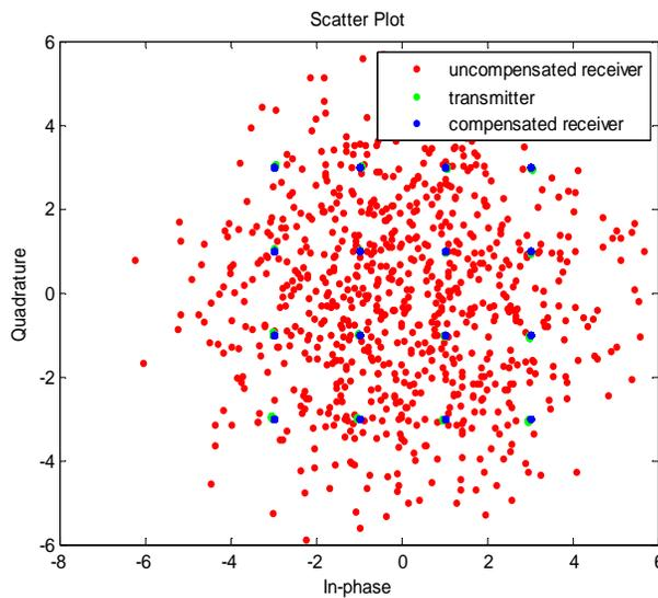
Figure 4.6 : Scatter plot of compensated received signal
