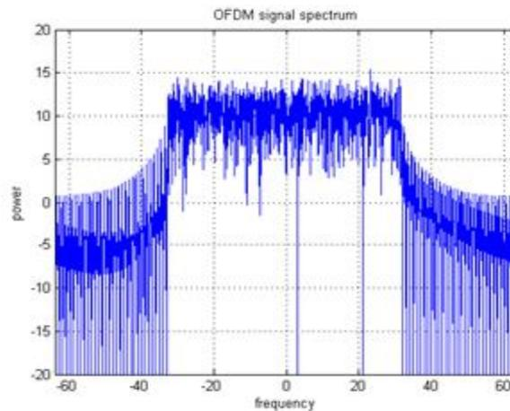
Figure 4.1: OFDM signal spectrum
