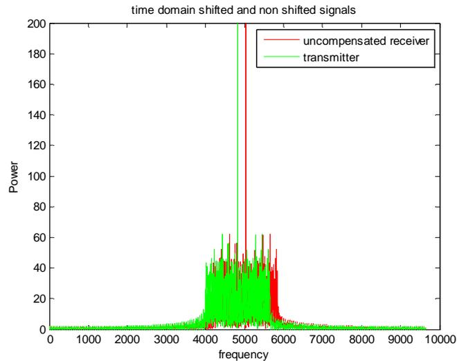
Figure 4.3 : Transmitted and received signal spectrums
