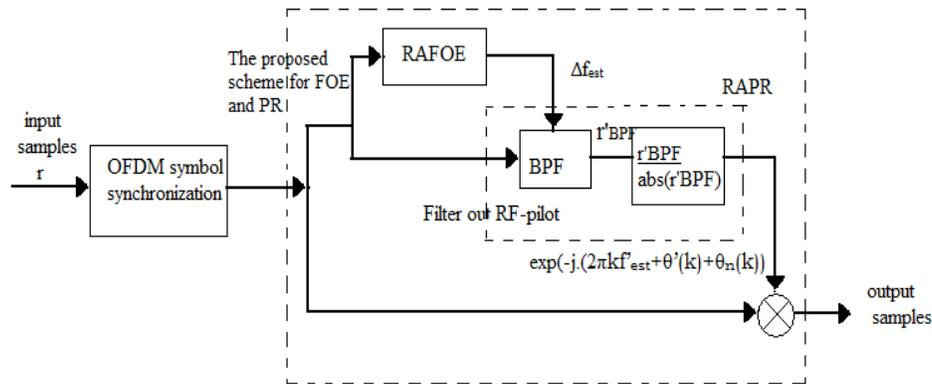
Figure 3.3: The block diagram of the proposed frequency offset and phase noise compensation
