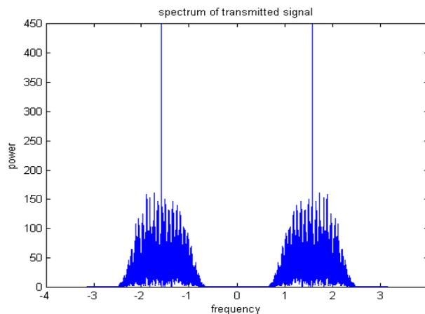
Figure 4.2 : RF-pilot carrier inserted OFDM signal spectrum
