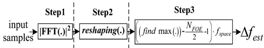
Figure 3.2: The block diagram of the RAFOE algorithm
