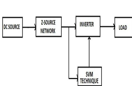
Fig. 1. Schematic of Z-Source inverter
