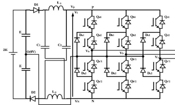
Fig. 2. Circuit of an REC Z source NPC inverter.
