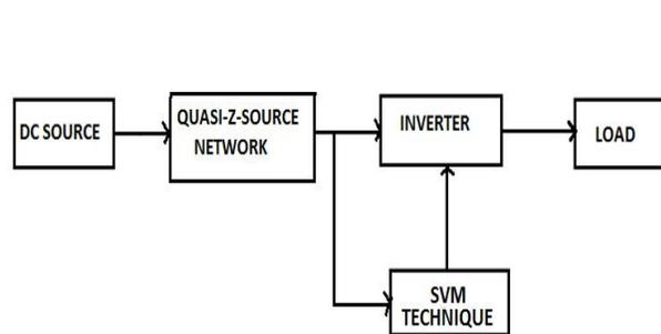
Fig. 3. Structure of the proposed quasi Z source inverter.
