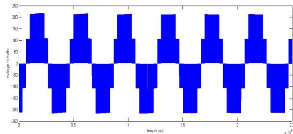
Fig. 12. Quasi Z source inverter output voltage waveform
