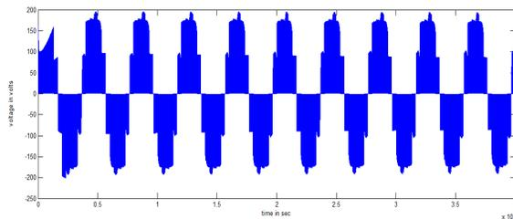
Fig. 8. conventional Z - source output voltage waveform
