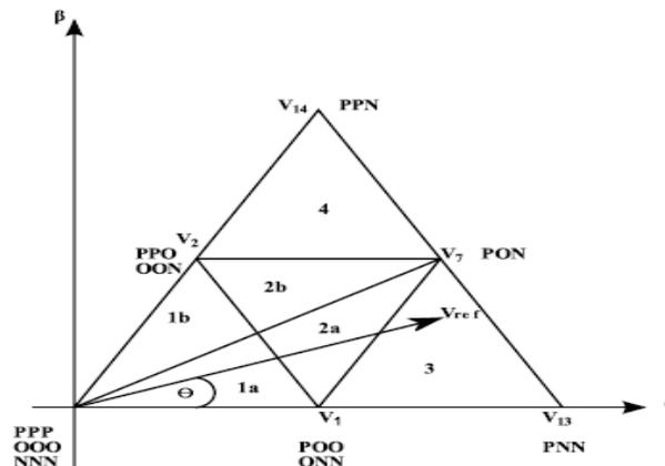
Fig. 7. Space vector diagram of a three-level inverter
