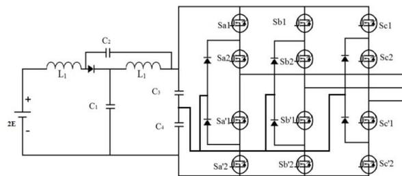
Fig. 4. Circuit of an quasi Z source NPC inverter
