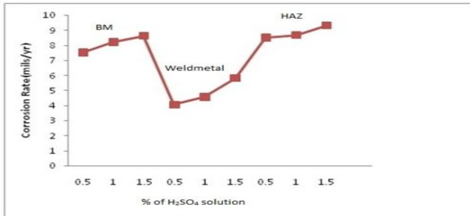
Fig 13 Representation of Corrosion Rate for various concentration of H 2 SO 4 solution
