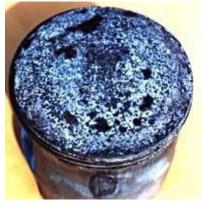
Fig.3.Melting of piston crown [2]
