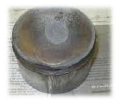
Fig.4Erosion on piston crown
