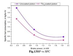
For the load applied for coated and uncoated piston revise of fuel consumption plays a important role in how efficient the work output is done for appropriated fuel consumption and utilization of that fuel as much as for combustion process. The graph shows a considerable decrease of fuel consumption for coated piston for the same load parameters of uncoated piston.
