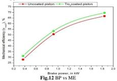
Efficiency is get increased as 6-7 % for the  $TiO_2$  coated piston when compared to uncoated piston for the change in pressure of 900  $lb/in^2$
