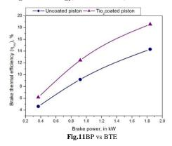
The graph shows start with good increase in efficiency with added brake power .This results that the change in pressure leads to a pop of 5% with increased load with constant speed. Variations are seen overview for the mechanical efficiency and get noted the amount of fuel consumed for the applied load.
