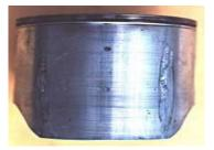
Fig.2.Four corner seizure on piston [2]
