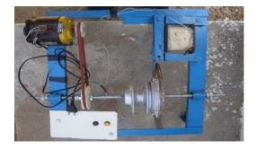
Fig 11 .Top view of the Fabricated Brake System
