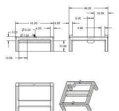
Fig. 5 Diagrammatic Representation of the Frame using Pro E Software
