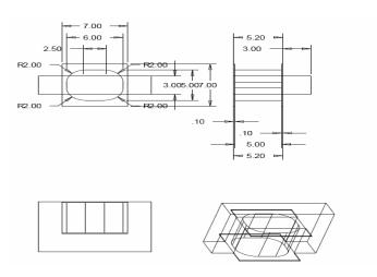
Fig.6 Diagrammatic Representation of the Electro Magnet using Pro E Software
