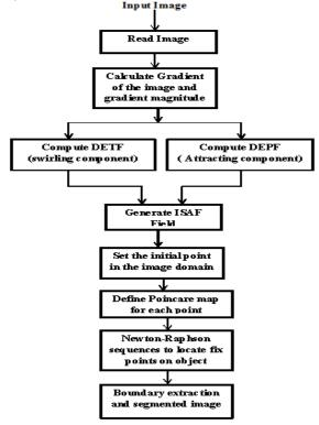
Fig: Block diagram of Boundary Extraction using Poincare map method
