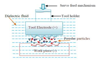
Figure 1: Principle of PMEDM Process
