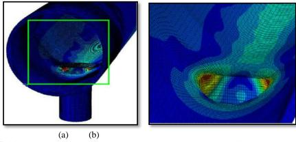
Fig. 2. (a) Von Mises equivalent stress distribution (b) Zoom image of equivalent stress. [6]
