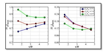
Fig. 5. Mean and fluctuating components of centreline velocity. [3]
