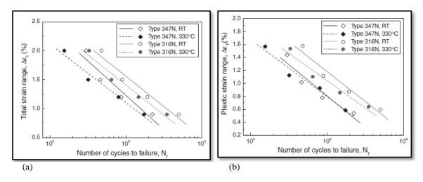
Fig. 6(a) Total strain range Vs number of cycles to failure(b) Plastic strain range Vs number of cycles to failure. [9]
