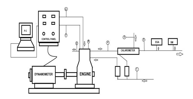
FIGURE3.1(1)WATER INLET TO THE CALORIMETER AND ENGINE  $(T_1^0C)$ ,(2)WATER OUTLET FROM THE ENGINE JACKET $(T_2^0C)$ ,(3)WATER OUTLET FROM CALORIMETER $(T_3^0C)$ ,(4)EXHAUST GAS INLET TO CALORIMETER $(T_4^0C)'$ (5)EXHAUST GAS OUTLET FROM THE CALORIMETER $(T_5^0C)$ ,(6)ATMOSPHERIC AIR TEMPERATURE $(T_6^0C)$ ,(7)FUEL FLOW,(8)PRESSURE TRANSDUCER. EGA: EXHAUST GAS ANALYER,SM : SMOKE METER,PC: PERSONAL COMPUTER
