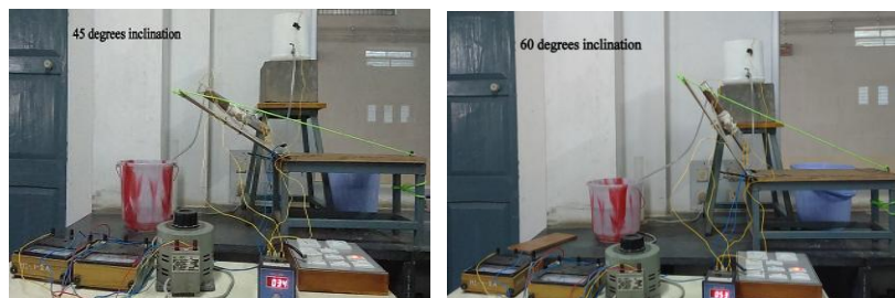
Fig.6. Readings noted from ammeter and voltmeter Fig. 7. Example of 45° and 60°inclination of square heat pipe while experiment is in process
