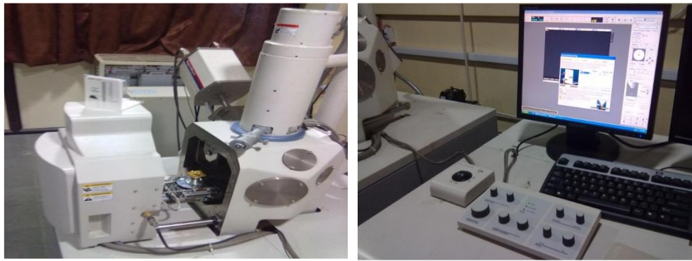
Figure 3.Loading and Magnification of the insert by use of S-3400N Scanning Electron Microscope
