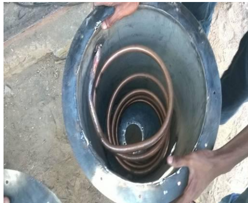
Fig.3 Copper tube inserted in cylinder
