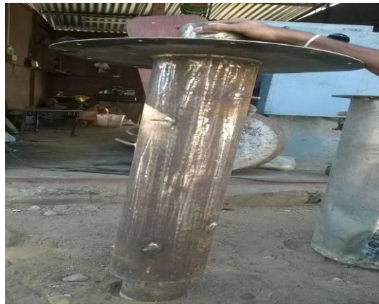
Fig.1 Exhaust gas flow pipe with copper fins
