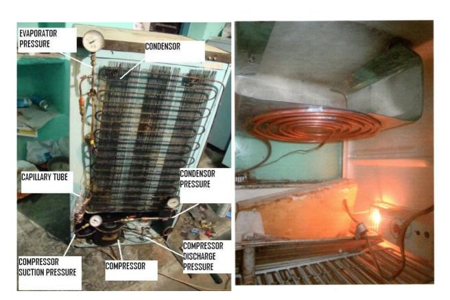
Fig. 4. Pictorial back view of the experiment
