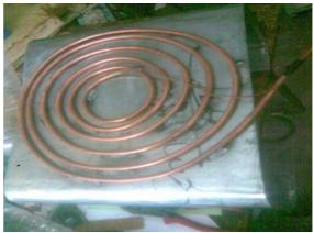
Fig.3. Ellipse Shaped Evaporator Coil
