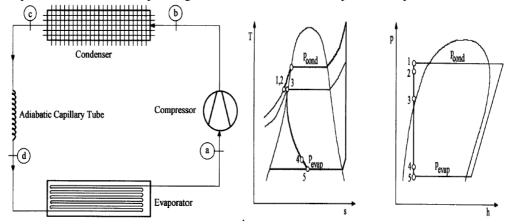
Fig. 1.1 Schematic diagram of vcr
