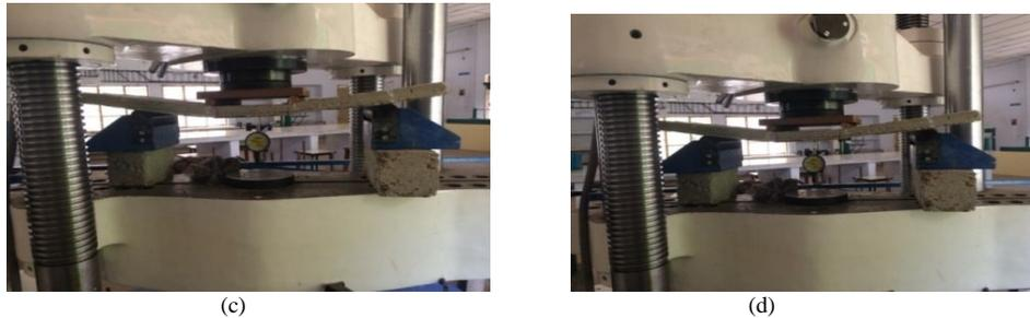
Fig. 4 (a) 28 days cured and dried specimen arranged for flexural test (two point load) (b) Applying load in small increments (c) loading of specimen to attain initial crack and corresponding dial gauge reading are measured at mid span (d) Loading continued till ultimate failure load situation has reached and corresponding dial gauge are measured at mid span for deflection
