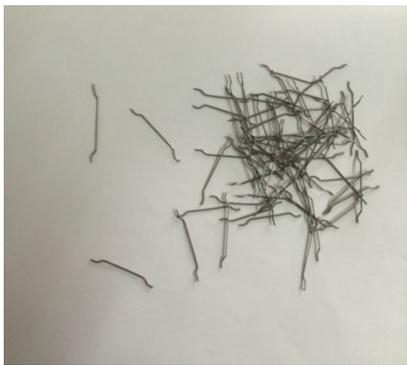
Fig 1 Hooked end steel fibers
