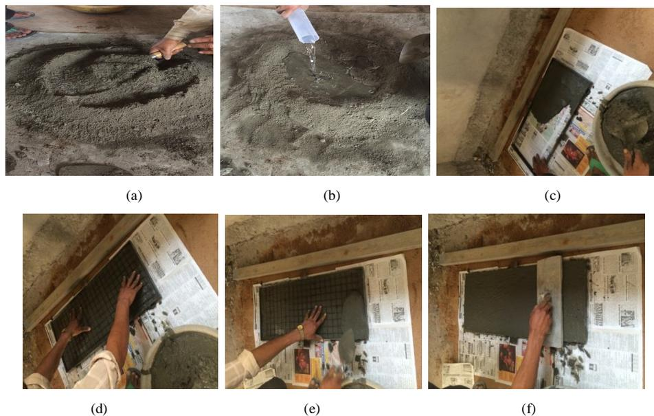
Fig. 2 Casting of specimens(a) Mixing of dry cement mortar uniformly with the addition of fibers (b) Addition of calculated amount of water to the dry mix (c) Laying of first layer of fibrous mortar in steel mould of thickness 11mm (d) Placing of welded mesh over the 1<sup>st</sup> fibrous mortar in the steel mould (e) Laying of second layer of fibrous mortar over the welded mesh of thickness 11mm (f) Finishing and smoothing of the top layer with help of trowel and screen board
