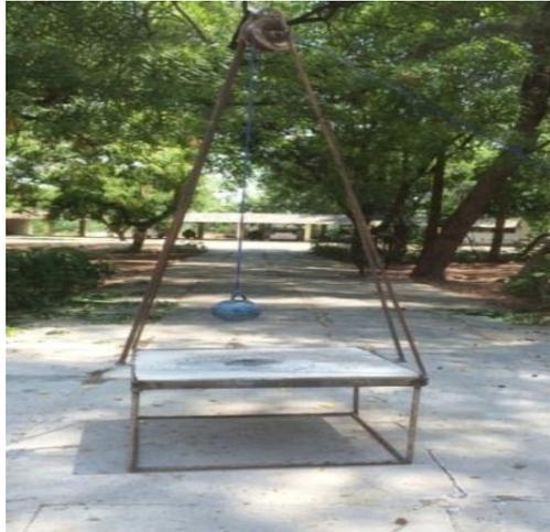
Fig 3 Impact test apparatus with pulley and steel ball arrangement
