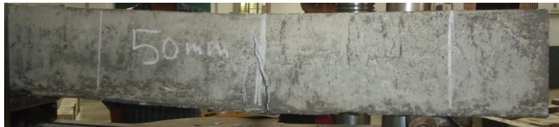
Figure 7: Failure of beam HCB-2
