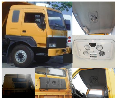
Fig.3Prototype evaporative air conditioner system with roof top unit fitted in conventional trucks
