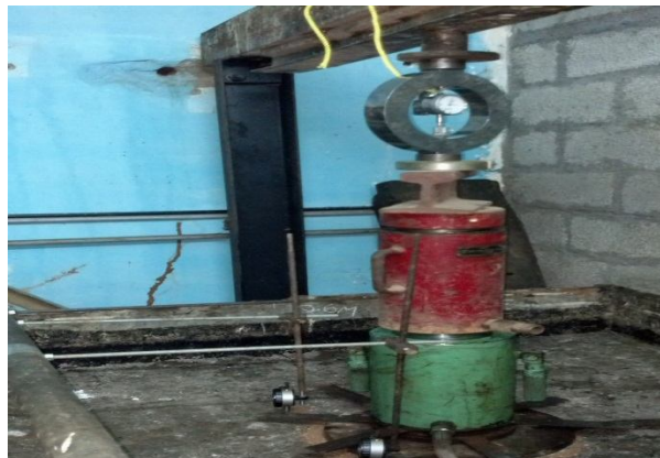
Fig-1: Model box setup with datum frame, proving ring and dial gauges
