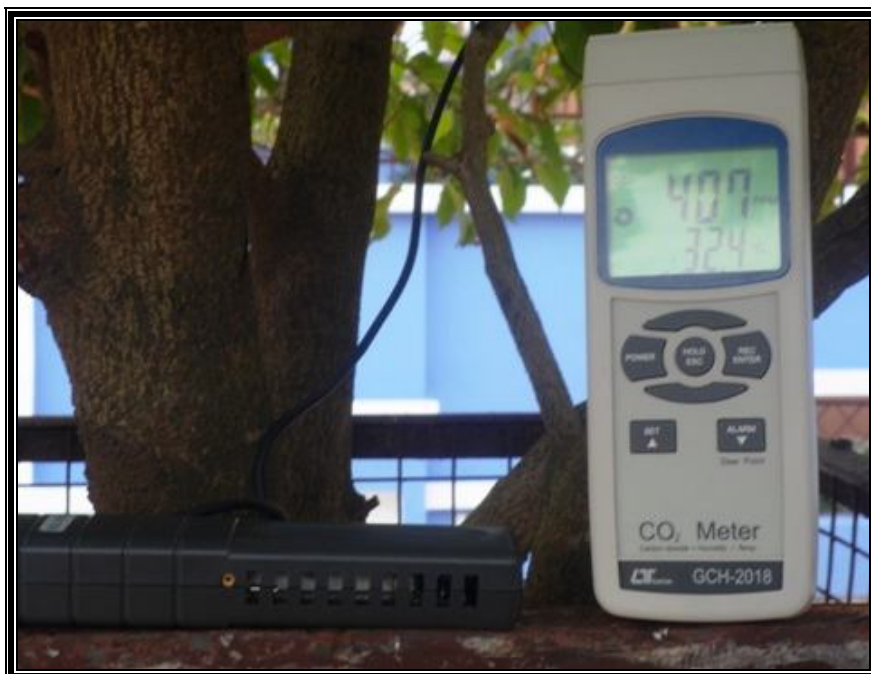
Figure 3: CO 2 analyser monitoring atmospheric carbon dioxide in the heart of the Bhubaneswar city
