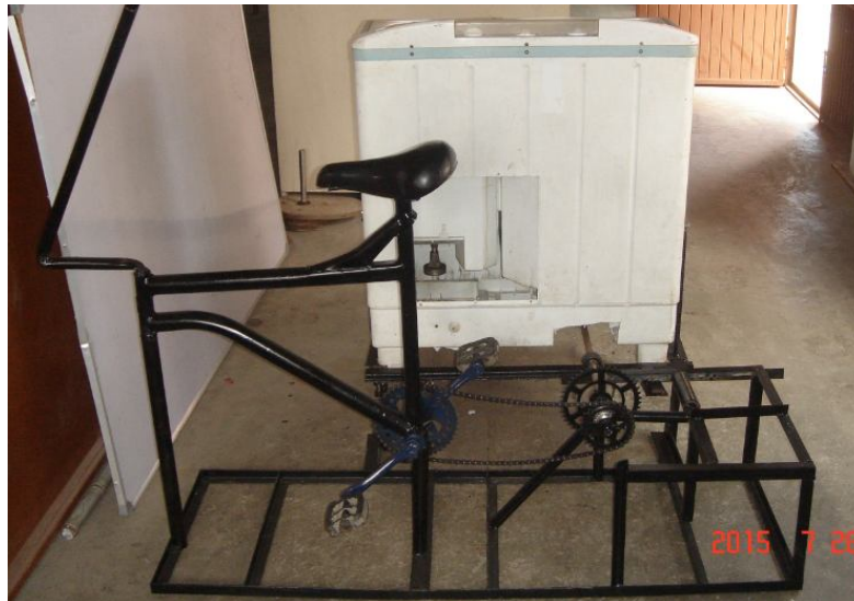
Figure 6. Assembly of pedal operated top loaded washing machine.
