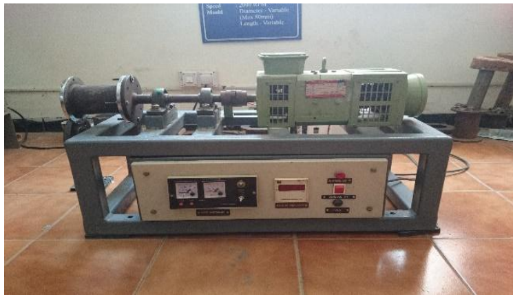
Figure 1. Experimental set up for Centrifugal casting
