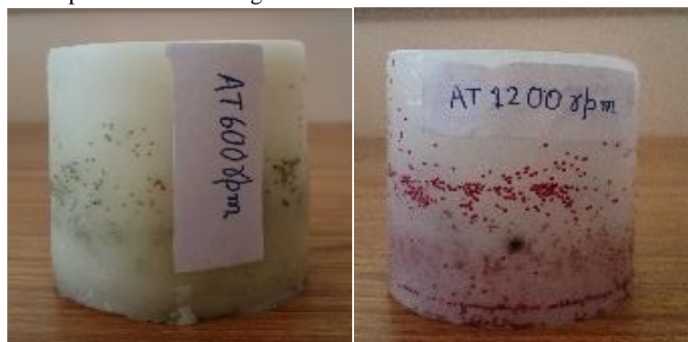
Figure 2.Cast of 5mm thickness obtained at different speed
