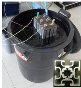
Fig. 4. Test layout during experimental investigation of thermal storage ability of PCM using heat exchanger made of aluminium profiles.
