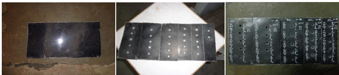
Figure 5 Results on RCFRP composite at different Pressure, AFR, and SOD, Nozzle diameter before and after machining
