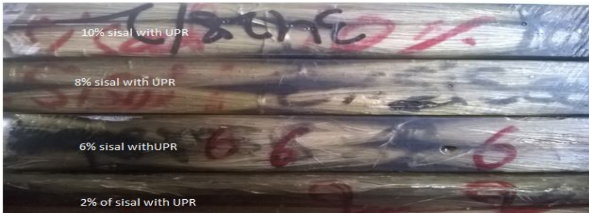
Fig 1: Unsaturated Polyester Resin (UPR) reinforced with sisal fiber
