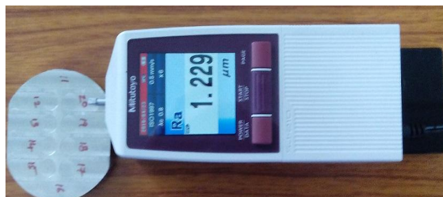
Fig.7 Measuring Surface Roughness R_a with Surf test Apparatus
