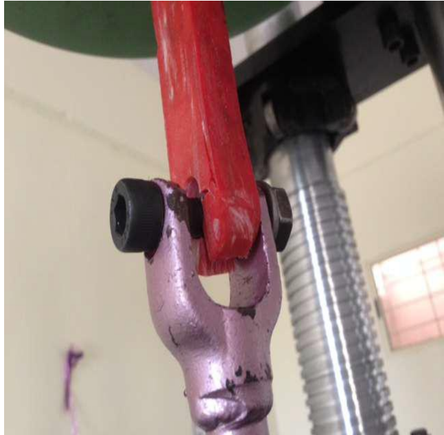
Figure 6.3 Failure Of Glass Fiber Link
