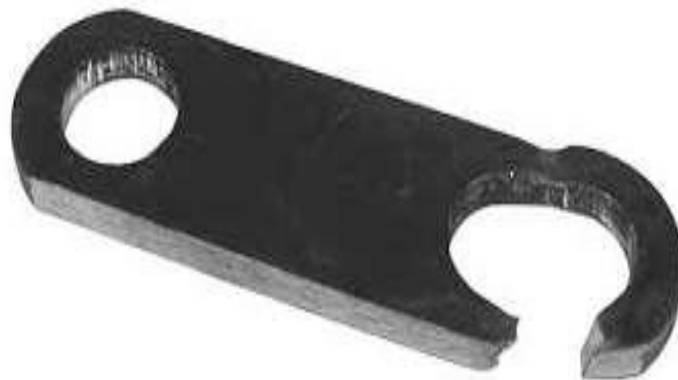
FIGURE 2.1 Failure of link
