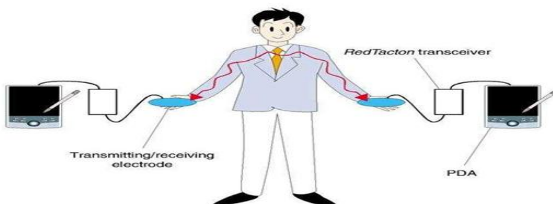
Fig.6 Experimental setup of Red Tacton
