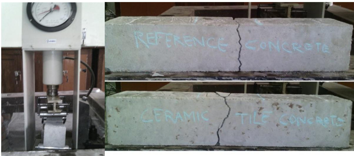
Figure -8: (a) Flexural strength testing apparatus with specimen (b) specimen after failure
