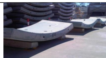
Fig 1.3 Earth Friendly Concrete (EFC) is a proprietary geopolymer concrete developed in Australia and used in a range of precast and in-situ applications .(2014)
