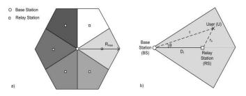
a)Hexagonal cell b)User location (rooftop mode Fig1: System model for a 6-sector urban cell
