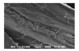
Figure 6a SEM micrographs of untreated fabric (C)
