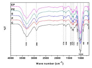
Figure 4. FTIR spectra of untreated (control, DC oxygen Plasma (P), PE, EP treated cotton fabrics
