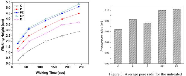
Figure 2. Wicking rate of DC oxygen Plasma (P), enzyme (E), PE and EP treated cotton fabrics
