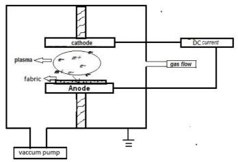
Figure 1. Schematic diagram of DC plasma Chamber
