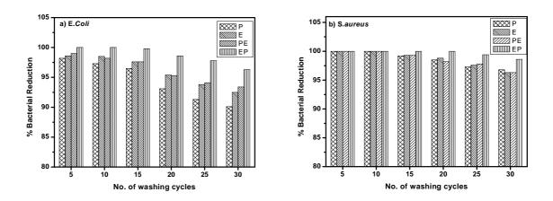
Figure 8. Wash durability of treated and untreated fabrics
