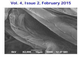
Figure 6 e SEM micrographs of EP treated fabric
