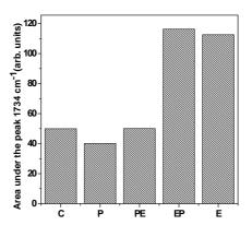
Figure 5. Area of 1734 cm<sup>-1</sup> peak of DC oxygen plasma and enzyme treatments
