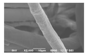
Figure 6c. SEM micrographs of cellulase enzyme treated fabric (E)
