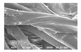
Figure 6d. SEM micrographs of PE treated fabric
