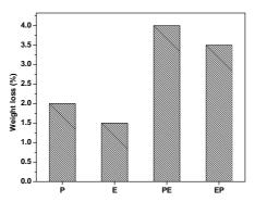
Figure 7. Percentage weight loss of Plasma (P), enzyme (E), PE and EP treated fabrics
