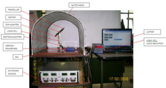
Fig. 4. Test bench 1 hardware
