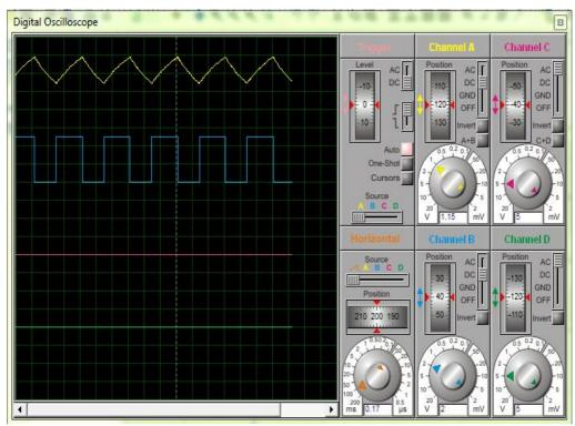
FIG 5 BOOST CONVERTER WAVEFORM, When the circuit was checked using digital oscilloscope on Proteus Software, these waveforms are obtained.
