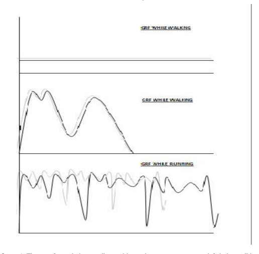
**Fig 1. GRF waveforms**. 1. The waveforms during standing position, when no power generated, 2 during walking when 5V approx generated and a single waveform is obtained and 3, the waveform during running when more than 5V is obtained thus giving double spikes.
