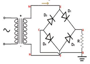
FIG 3. BRIDGE RECTIFIER
