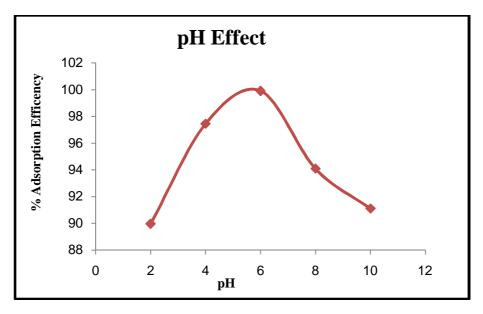
**Figure 3** Effect of pH on the adsorption efficiency of  $Cr^{3+}$  onto MWCNTs.
