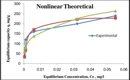
Figure 4 Adsorption isotherms of experimental and theoretical models of MWCNTs (25°C and 25mg).
