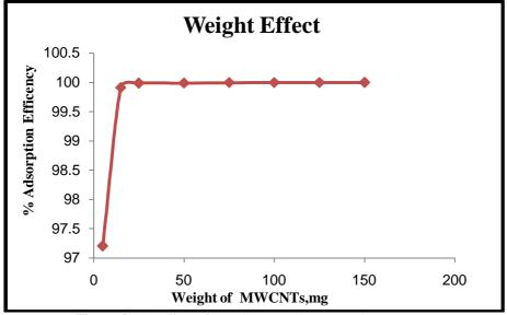
Figure 2 The effect of MWCNTs on the adsorption process.
