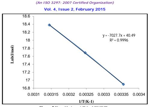
Figure 5 Plot of Lnb vs. 1/T for MWCNTs.
