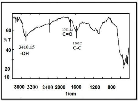
Figure 1 FTIR of Functionalized multi wall carbon nanotubes.
