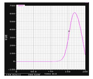
Fig 12.FBCM powerThe power wave is obtained for modified FBCM, shown in Figure 4.19 which implies the decrease in power dramatically after a sudden rise, thus this modified circuit uses less power to be used.
