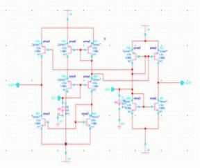
Fig 6 Fully balanced current mirror
