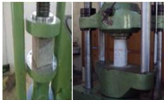
Fig 3. Testing of Cube and Cylinder
