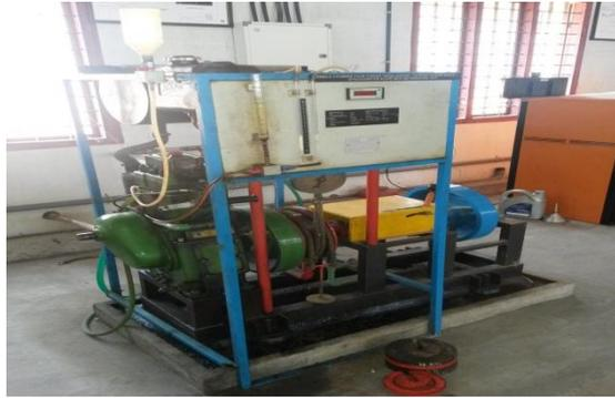
Fig 1.1: Kirloskar Engine with Mechanical rope brake drum dynamometer.
