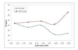
Fig7. Variation of hydrocarbon with brake power
