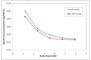
Fig2. Variation of specific fuel consumption with brake power
