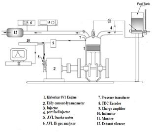
Fig1. Experimental setup of Kirloskar SV1 Engine
