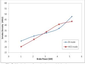
Fig5. Variation of particulates with brake power
