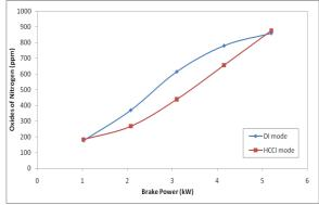
Fig4. Variation of oxides of nitrogen with brake power
