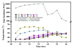
Fig 3: Heating curves of the heat exchangers (TT-pipe temperature), PCM (TP-paraffin temperature), HTF.
