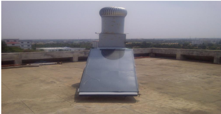
Figure 1: Experimental Setup of a solar Flat Plate collector.
