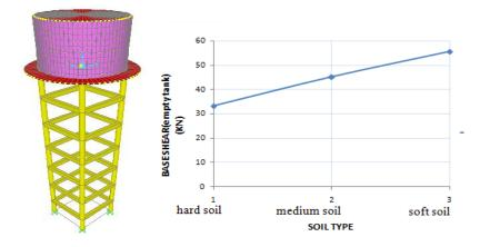
Figure 5.1 SAP2000 Model of elevated water tank. Fig 5.10 soil type vs. base shear
