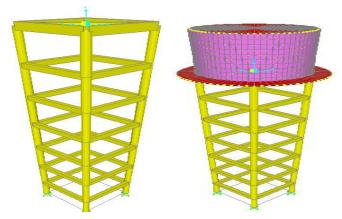
Figure 4.2 Frame of the water tank staging.
