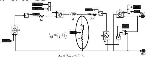
Fig.2 Equivalent Circuit on d Axis without Damper winding.
