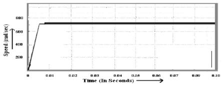
Fig. 24 Step Response of speed for ANFIS Controller
