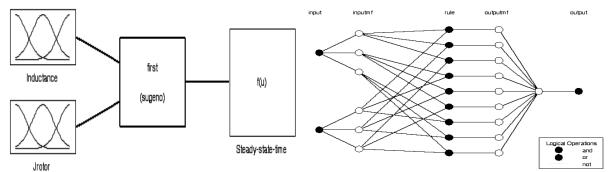
Fig.8 Fuzzy model of the synchronous motor.
