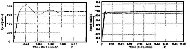
Fig. 18 Response at speed of 650 rad/s with ANFIS Controller
