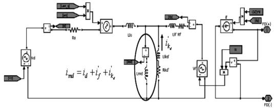
Fig3. Equivalent Circuit on d Axis with Damper winding
