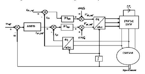
Fig. 7. System Configuration of Field-Oriented CSI fed Synchronous Motor (CSIFSM) Control
