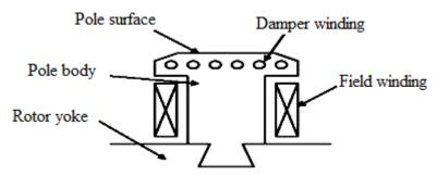
Fig.1 Salient Pole Rotor Construction
