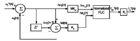
Fig.8. Fuzzy speed controller Construction
