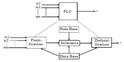
Fig. 4 The internal configuration of a fuzzy logic Controller
