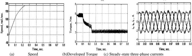
Fig.10. Simulation starting responses of the proposed Fuzzy based CSI fed Synchronous Motor (CSIFSM) drive at rated speed and rated load conditions.
