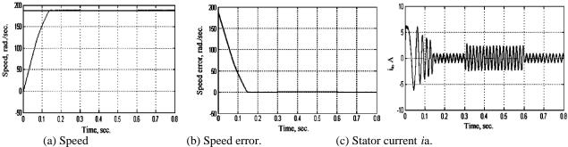
Fig.11. Simulation responses of the fuzzy based CSI fed Synchronous Motor (CSIFSM) drive for a step change in load...
