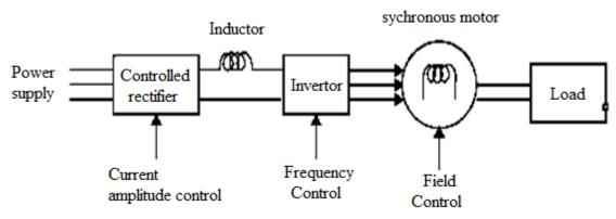
Fig. 1 Drive configuration for open-loop CSI fed Synchronous Motor (CSIFSM) control
