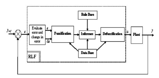
Fig.5 Basic structure of fuzzy control system
