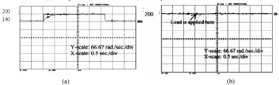
Fig.14. Experimental speed response of the fuzzy based CSI fed Synchronous Motor (CSIFSM) drive for (a) step change in speed and (b) step change in load.
