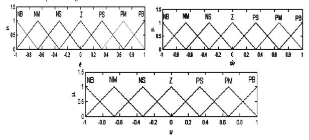
Fig.6. Membership functions for input e, de and u
