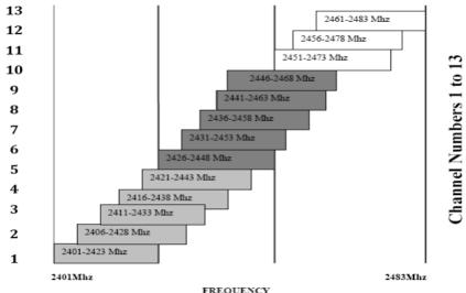
Fig. 1 IEEE 802.11 WLAN Frequency Spectrum
