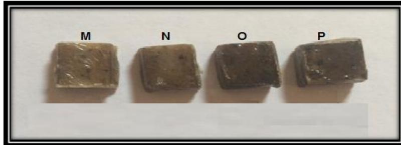
Fig. (5) RPET/ S.W.D composites with different melting temperature M-at 180 °C , N-at 200 °C ,O-at 220 °C and P-at 240 °C for Water absorption test
