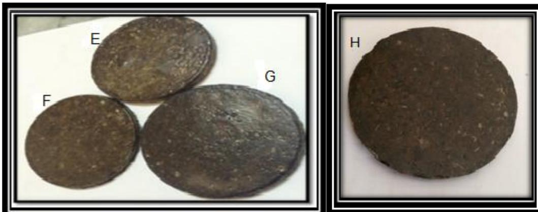
Fig (3) RPET/S.D.W composites with different melting temperature (E -at 180 °C, F -at 200 °C, G-at 220 °C and H-at 240 °C) for thermal conductivity test .
