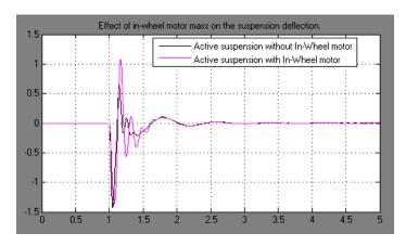
Fig. 8 Effect of IWM on the suspension deflection
