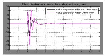
Fig. 12 Effect of IWM on the acceleration of sprung mass.
