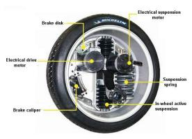
Fig. 2 Michelin active tire with In-Wheel Motor.
