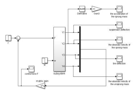
Fig. 7 Simulink model of active suspension system with controller.
