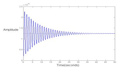
Fig. 6 Open-Loop Response to 0.1 m Step Disturbance of active suspension system
