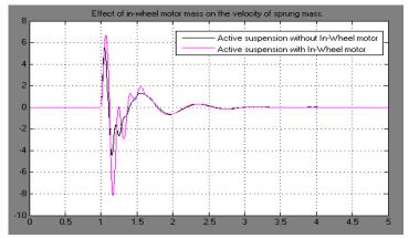
Fig. 10 Effect of IWM on the velocity of sprung mass.
