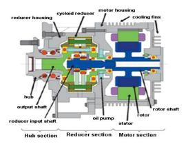
Fig. 1 Two Cross-section of In-Wheel Electric Motor.
