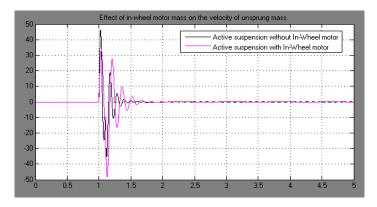
Fig. 11 Effect of IWM on the velocity of unsprung mass
