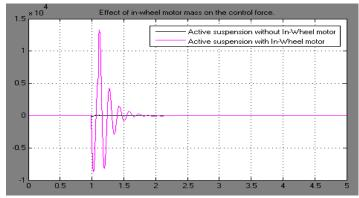
Fig.13 Effect of IWM on the control force F.
