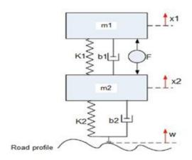
Fig. 4 Double Mass-Spring-Damper used to model Active Suspension system.
