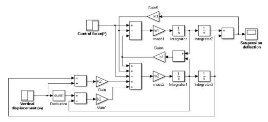
Fig. 5 Simulink diagram of active suspension system.
