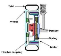
Fig. 3 Bridgestone's Dynamic-Damping In-Wheel Motor Drive System.
