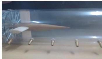
Fig. 5.4: Smoke flow visualization
